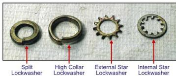
Lockwasher are not used on structural connections and connections where bolts are torqued. All lockwashers are sized by the nominal dimension of their internal diameter.
