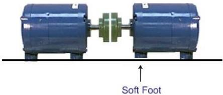
have two soft-feet. If not corrected prior to tightening down the mounting bolts, this condition will cause machine frame strain, resulting in another form of misalignment called internal misalignment. This condition will most likely result in accelerated bearing wear and possible shaft failure.
