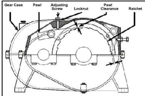
designs may vary, the brakes work on a similar principle. Two or more friction surfaces are held tightly together when a load is lifted by the action of a screw (helix) or an inclined plane. This type of brake commonly uses a ratchet and pawl mechanism or a sprag clutch for holding the centermost friction plate stationary when the load is lowered.
