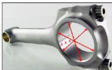
this method, the crane mechanic will be able to determine whether the bearing has elliptical or taper alignment issues to correct. Before installing the bearing in a bore, the bore should be checked in a similar manner, as any irregularity in the bore will be transferred to the bearing.
