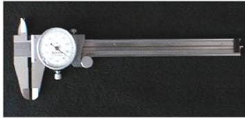
Electrolysis may result, damaging the jaws. Wiping the caliper down after use is good practice to clean and prevent corrosion. Don't try to get a reading by using excessive force on the jaws. The consequence will be an inaccurate reading and possibly a damaged tool.
