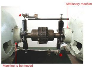
For horizontal readings, looking toward the stationary machine, zero the "A" dial at the 3 o'clock position, and zero the "B" dial at the 9 o'clock position. No compensation for indicator sag is needed at the 3 o'clock and 9 o'clock positions since the movement of the indicators in this position will not affect the readings.
