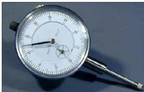
usually in thousandths, but can be as small as 50 millionths of an inch. Travel range can be from .003" to 12", but normal travel ranges are 1/4", 1/2" and 1". Dial indicators may be fitted with a variety of tips for special applications and are normally used with a stand allowing the operator to position them in correct orientation to take the reading.
