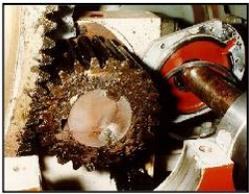
Misalignment causes vibration and machine strain which can destroy critical parts of the machine such as bearings, seals, gears, and couplings. Failures of this type are usually evident, although often mistakenly identified as "normal wear and tear". To lessen the chance of failures, it is important for the crane mechanic to properly set up and align equipment.
