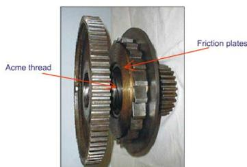
**MAIN SECTION OF MECHANICAL LOAD BRAKE: MOTOR GEAR**
