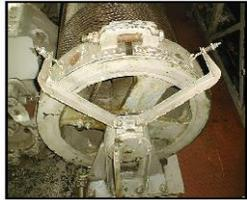
disassembled to inspect linings for wear, de-bonding, or glazing. Brake drum surfaces should be inspected for smoothness and for evidence of overheating. The proper alignment of brake shoes and adjustment settings should be verified. Inspect brake linings for significant wear, which may cause rivets to contact the wheel, and uneven wear, which can be a symptom of improper mounting, worn parts, or improper adjustments.
