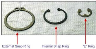
Reduced cross-section external E-rings, contain three prongs connected by a reduced section bridge to provide greater resilience during installation. They are installed radially, usually by means of an applicator, and provide a high shoulder for abutment by a retained part. Snap rings are normally identified according to a size chart.
