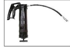
contaminants. When changing types of grease in a grease gun, all of the old grease should be removed first. Do not forget to purge the hose by pumping some grease through it before using the gun on equipment. When filling a grease gun with grease, be sure to label the gun with the proper NFPA information to identify the grease contained in it.
