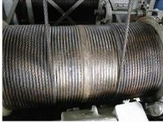
During operation verify in all operating conditions, including extremes of hook or boom positions, that no less than two complete wraps of wire rope remain on grooved drums and at least three complete wraps remain on smooth drums.
