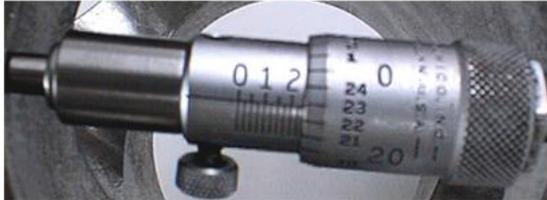
2. Read the depth micrometer depicted below and give the measurement. The rod in the mic is a 0-1" rod.
