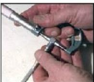
the gauge’s telescoping rod to expand against the sides of the hole. Gently tighten the lock keeping the handle at a slight angle. Next, position the handle to the upright position (parallel to the sides of the hole) and carefully remove from the hole, ensuring the gauge’s lock is sufficiently tightened. Now, using an outside micrometer, the inside diameter of the hole can be determined.
