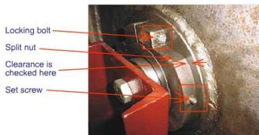
backing off the split nut and checking the clearance between the nut and the motor gear. There must be sufficient clearance so that the plates can unscrew when the motor is turning in the “lower” direction, but not so much that when they screw back together the force will lock them together.
