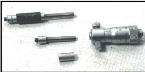
micrometer only has a 1/2" range or travel. Once the pieces have been selected, the micrometer must be assembled. The spacer should be slipped over the rod, and then the rod inserted into the micrometer head and the clamping screw tighten. On some instruments, there are match marks on the rod and the micrometer head for orienting their position.
