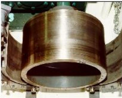
section of the lining, overheating of the lining and, if not remedied, a reduction in brake performance. Many of the new synthetic lining materials are susceptible to burning, so it is important that the arcing be performed correctly. The final determination as to whether a brake lining has adequate contact area is the brake's ability to support a test load. Keep in mind that there are other factors such as the force exerted by the torque spring which can also affect the brake's performance.
