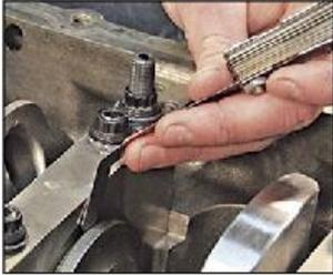
a blade based on an estimation of the clearance to be measured and carefully try to engage the blade in the opening. If the blade fits easily, the next larger size should be tried. If the next larger size fits, without excessive force, the next larger size should be tried. Repeat this process until a blade fails to fit and then go back to the previous blade. Do not force blades.
