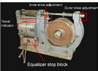
centered above the equalizer stop block. The travel indicator shows the mechanic or crane operator when the linings are worn to the point where re-adjustment is needed. When the ends of the indicator plates line up, the maximum gap has been reached, indicating re-adjustment is due. The brake equalization process is complete when both shoes have been equally adjusted to specifications.
